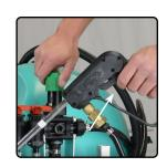
**10)** To maximize the life of your pump maintain pressure settings that do not cause the pump to pulsate whenever possible.
