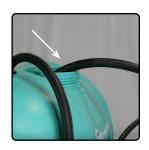
**6)** Connect the wire harness to the bullet connector at the pump.
