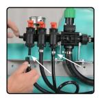
**4)** Before running your pump, make sure the regulator is fully open to avoid premature wear or damage to the pump.
