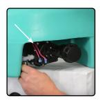
**4)** Hook the wire harness to the bullet connector at the pump.
