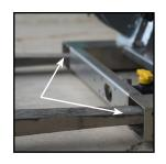
**2)** When loading your sprayer, we recommend placing a block of wood between your sprayer and the front of the bed of your truck.
