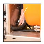
**6)** Connect the cables to the pumps. Make sure to plug in the correct connectors to the corresponding pumps as shown in this image.
