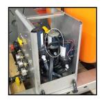
**14)** Simply unhook the hoses and exchange the pump hook ups.
