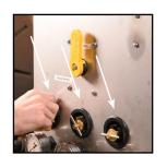
**4)** Switch the yellow handle to the horizontal position labeled as "boom spray".
