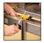
**13)** If you are experiencing trouble with your center lane pump while spraying, you can exchange it with one of the side discharge pump ports to continue spraying with your center lane.
