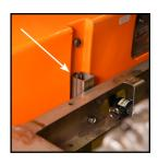
2) Tighten the hardware making sure the square neck on the carriage bolt is fully inserted through the slot.
