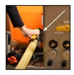
**9)** To use the spray gun, ensure the valve to the hose reel is in the open position.
