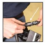
**8)** Connect the controller to the power cables.
