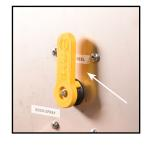
**10)** To clean your filter during use, twist the red insert clockwise and pull it out. This will engage a valve in the filter body to stop liquid from draining out the line.
