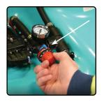
6) Squeeze the hand gun trigger to start discharge and then adjust the pressure to your desired setting while keeping the gun trigger engaged.
